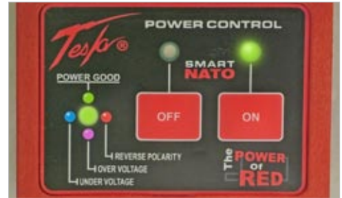
Figure 1: Status LED showing “ON” power good
