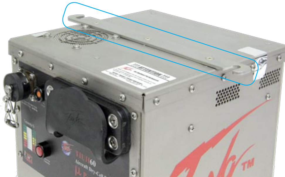
Figure 3.8.1 – Battery Lock-down (outlined in blue)
