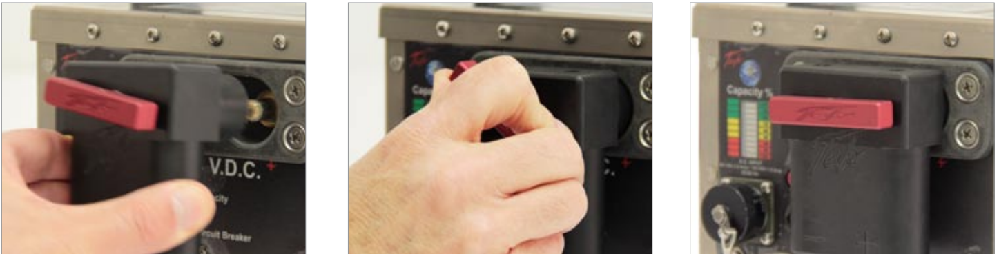
Figure 3.10.1 Attaching DC Power Cable to TIUH60 MPU-24
