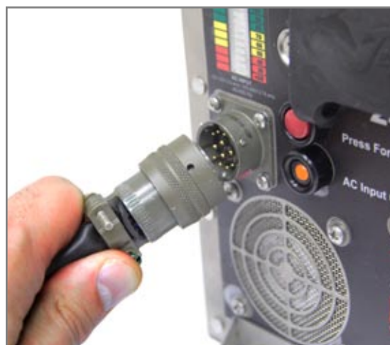
Figure 3.13.2 Attaching AC Line Cord
