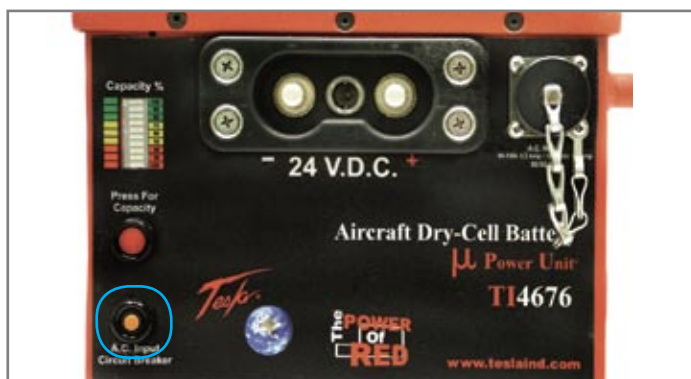
Figure 3.11.1 AC Input Circuit Breaker location (outlined in blue)
