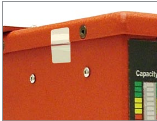
Figure 5.2.1 – Warranty Void stickers Front and Back on the unit
