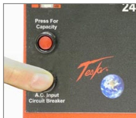
Figure 3.11.2 Pushing AC Input Circuit Breaker
