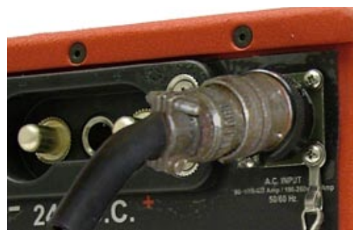
Figure 3.12.2 AC Input Line Cord Attached
