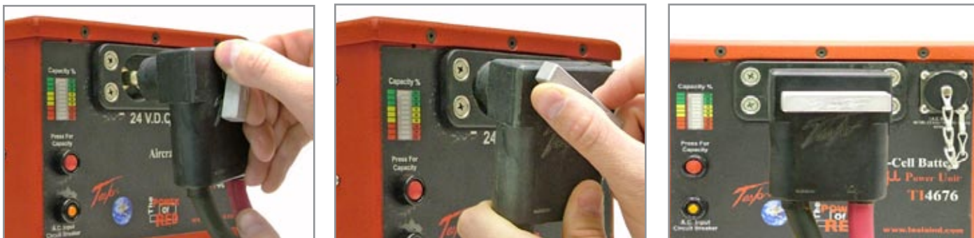
Figure 3.9.1 Attaching dc power cable to MPU
