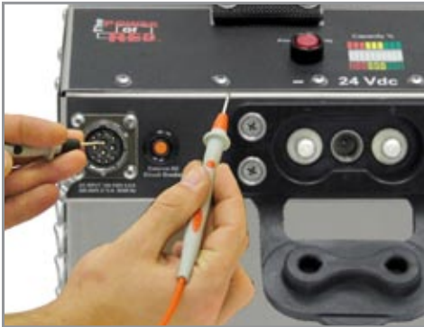
1. Place the negative probe on the ac ground probe ( J or L) and the positive probe on an exposed part of the metal case.
