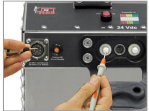
3. Move the positive probe to the dc negative post on the dc output connector.
