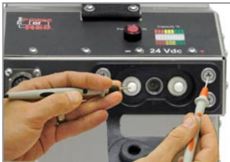
5. Move the negative probe to the dc negative post on the dc output connector.
