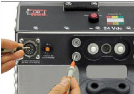
4. Move the positive probe to one of the four screws securing the dc output connector to the unit casing.
