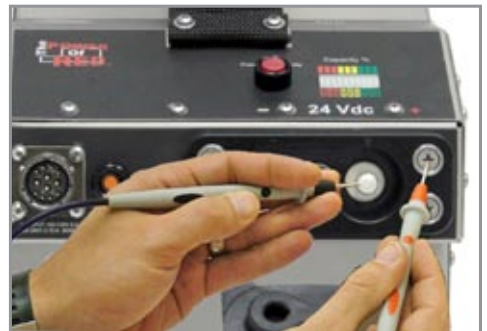
6. Move the negative probe to the dc positive post on the dc output connector.
