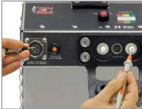
2. Move the positive probe to the dc positive post on the dc output connector.
