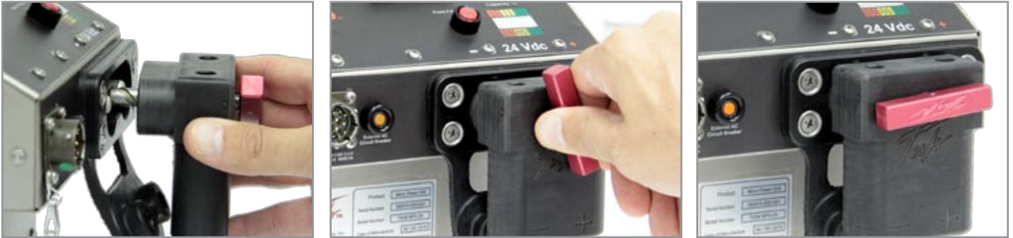
Figure 3.10.1 Attaching dc power cable to TI206 MPU-24
