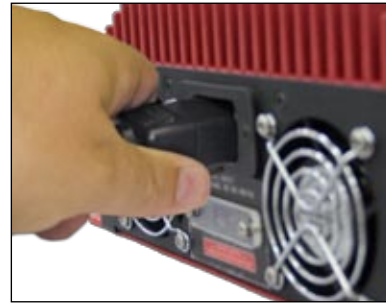
Figure 3.1.2 – Connecting AC line cord
