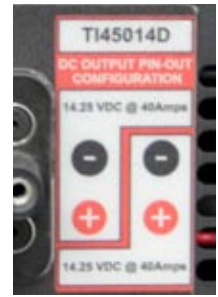
Figure 4.3.1 DC Output Pin-Out Configuration
