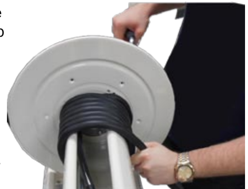
Figure 3.1.3 Wrapping the cable onto the reel
