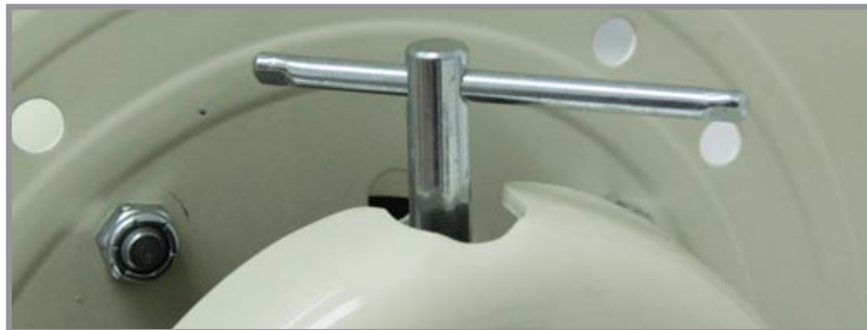
Figure 3.3.1 - Crank to adjust the reel drag.
