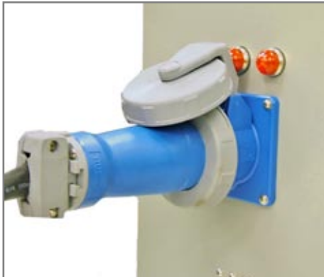
Figure 2.8.3 208 VAC cable plugged in.
