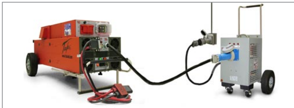
Figure 4.5.3 DC cable plugged into GPU.
