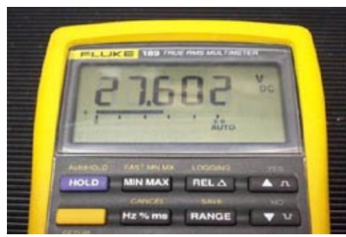
Figure 6.2.5 – Multimeter reading typical 24 V power cell voltage
