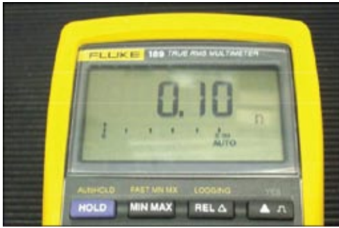
Figure 6.2.2 – Multimeter reading continuity
