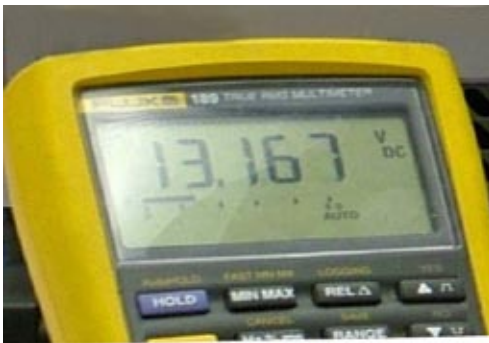
Figure 6.2.4 – Multimeter reading typical 12 V power cell voltage
