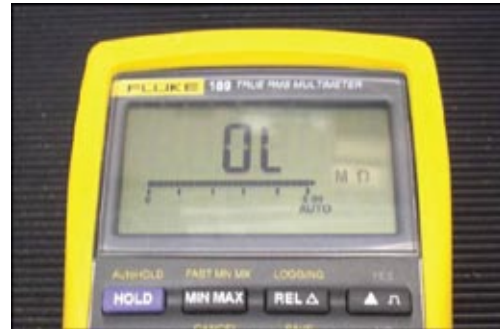
Figure 6.2.3 – Multimeter reading open circuit
