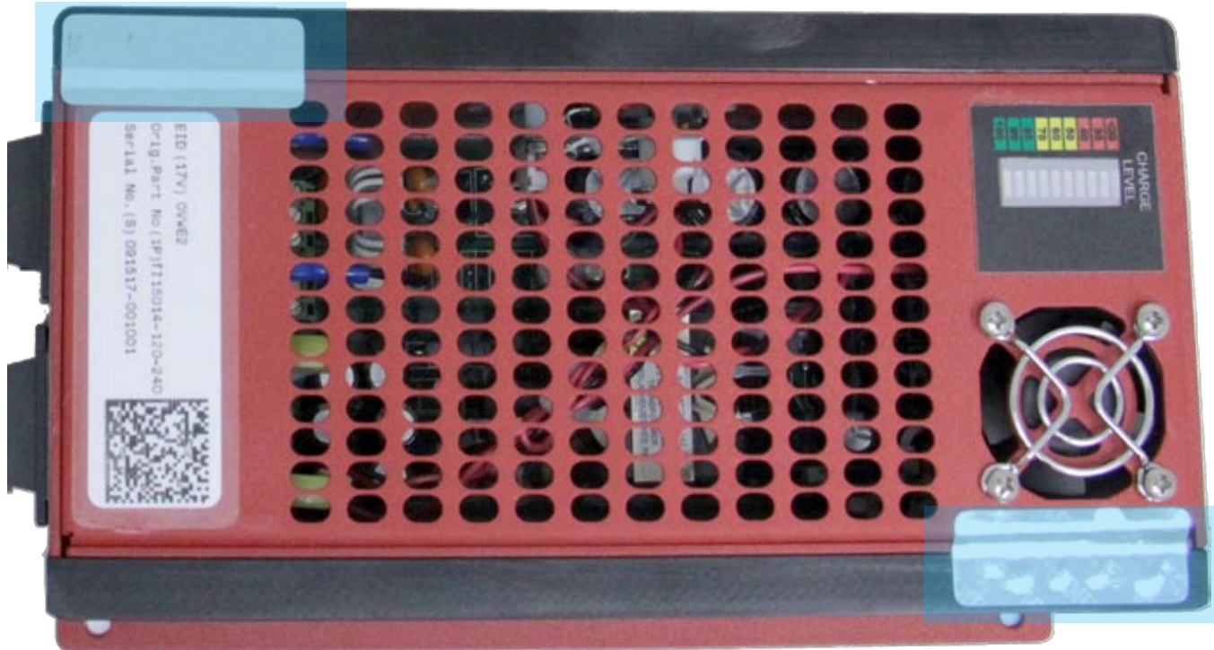
Figure 6.3.1 – Warranty Void Stickers (highlighted in blue)
