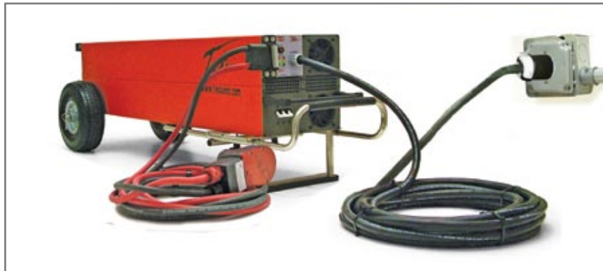
Figure 3.13.2 Connecting TI4200 GPU-24-PFC to AC Power Supply with DC Power Cable Attached
