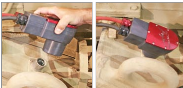
Figure 3.11.2 Attaching NATO DC Power Cable to vehicle
