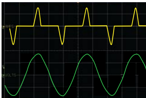
Figure 2.9.1 - Non-PFC Power Supply
