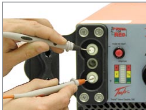
Figure 3.8.3 – Testing DC Receptacle
