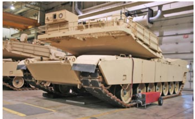
Figure 3.11.3 Starting vehicle with TI4200 GPU-24-PFC
