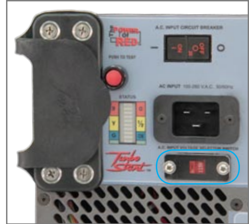
Figure 2.10.1 Input Voltage Selector Switch (outlined in blue)
