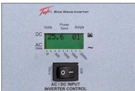
Figure 3.15.1 Inverter Display Panel with Switch set to “I” (ON) position.
