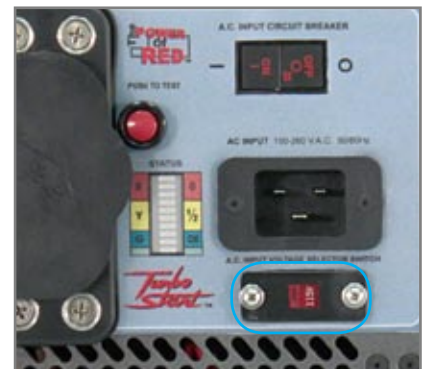
Figure 1.3.4 – TI3000 GPU-24-INV-1800 Input Voltage Selector Switch
