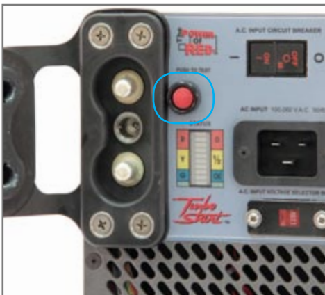
Figure 2.11.1 - “Push to Test” button location (outlined in blue)
