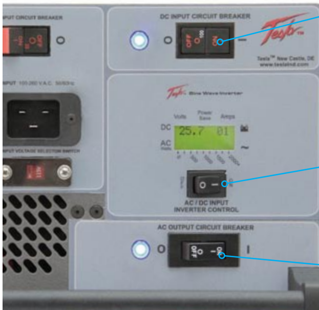
Figure 3.20.1 TI3000 GPU-24-INV-1800 with Inverter Activated
