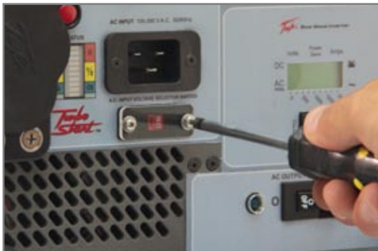
Figure 2.10.2 - Unscrew Protective Cover
