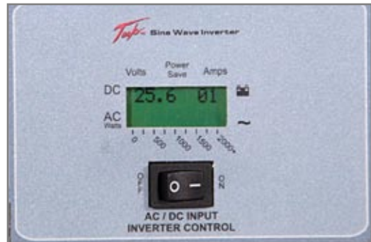
6.3.2 Inverter Display Panel and On/Off Switch turned on and active.
