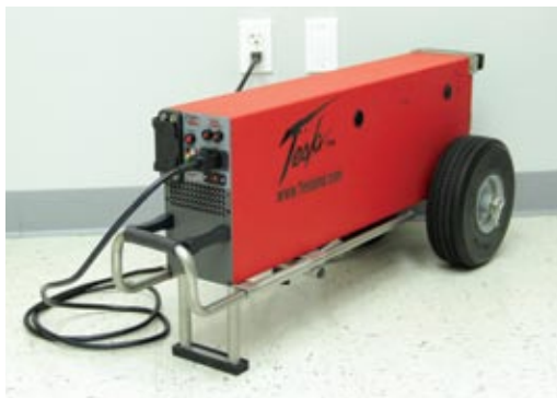
Figure 4.3.1 Connecting TI3000 GPU-24 to AC Power Supply
