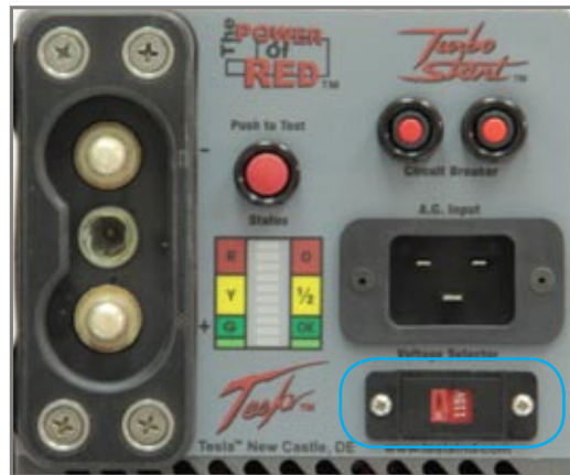
Figure 2.10.1 Input Voltage Selector Switch (outlined in blue)
