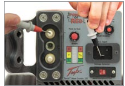
3. Move the positive probe to the dc negative post. Multimeter should read greater than 10 M \Omega .
