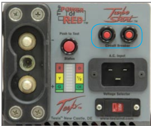
Figure 2.8.1 - AC Input Circuit Breaker (outlined in blue)
