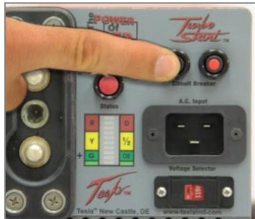
Figure 2.8.2 - Pressing Circuit Breaker
