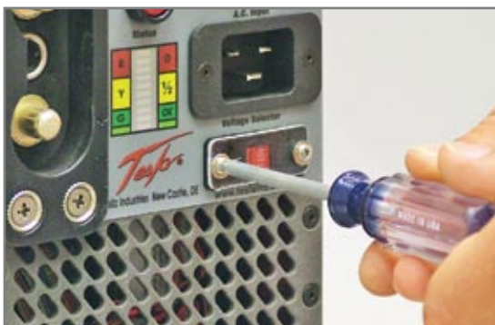
Figure 2.10.2 - Unscrew Protective Cover
