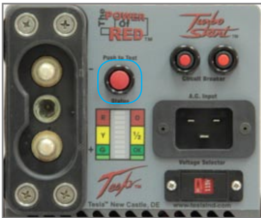
Figure 2.11.1 - “Push to Test” button location (outlined in blue)
