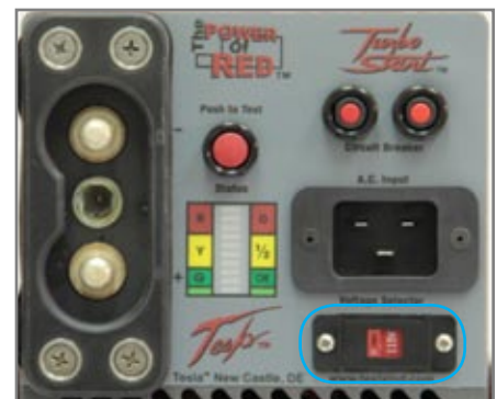
Figure 1.3.4 – TI3000 GPU-24 Input Voltage Selector Switch
