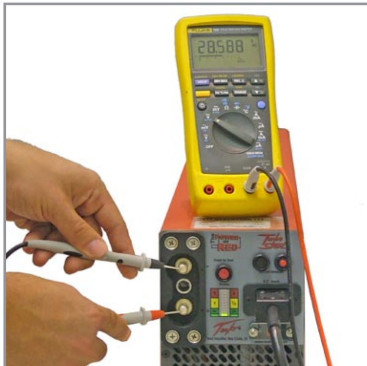
Figure 3.8.2 – Testing DC Receptacle
