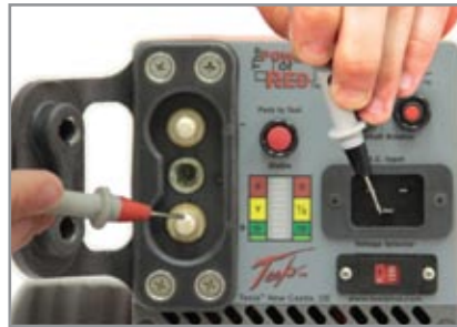
2. Place the negative probe on the ac ground post and the positive probe to the dc positive post. Multimeter should read greater than 10 M \Omega .
