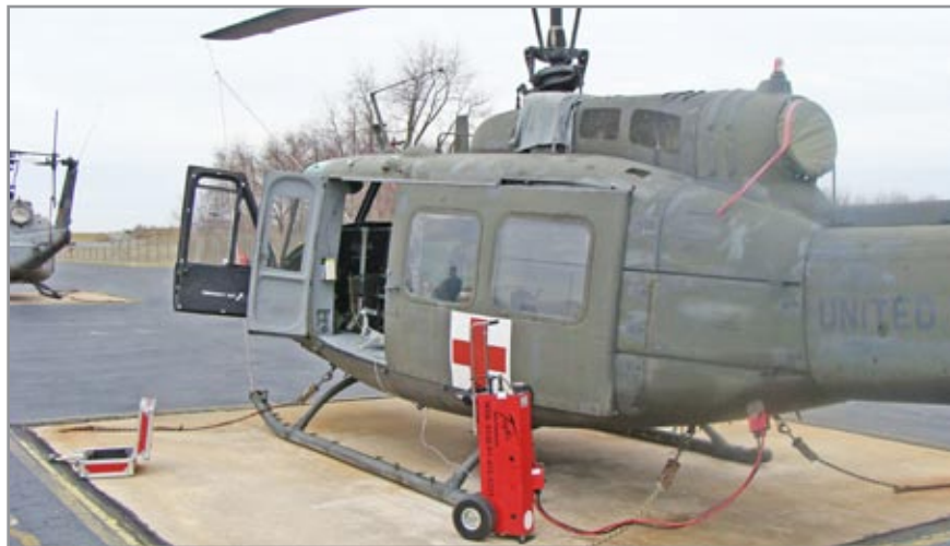
Figure 3.11.4 Starting UH-1 Huey Helicopter with TI3000 GPU-24
