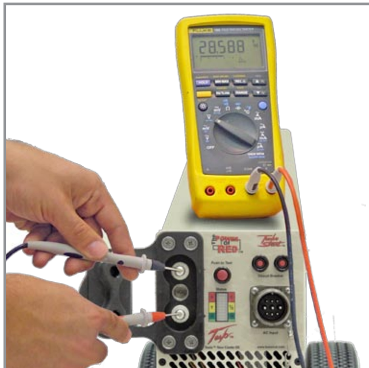
Figure 3.8.2 – Testing DC Receptacle
