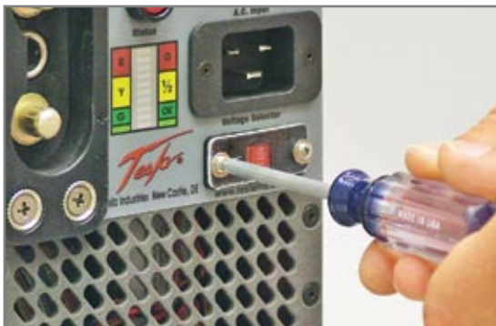
Figure 2.11.2 - Unscrew Protective Cover
