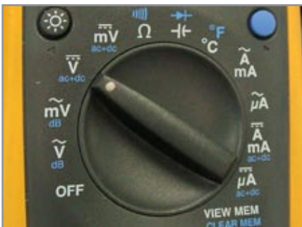
1. Set multimeter to Volts.
