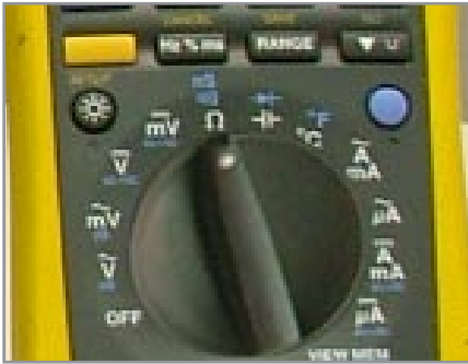
1. Set multimeter to Ohms.
