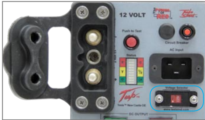
Figure 2.11.1 Input Voltage Selector Switch (outlined in blue)
