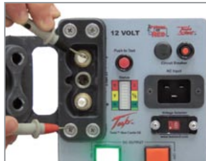
2. Place the positive probe to the fastener screw on the dc receptacle. Move the negative probe to the dc negative post. Multimeter should read 0 Volts.
