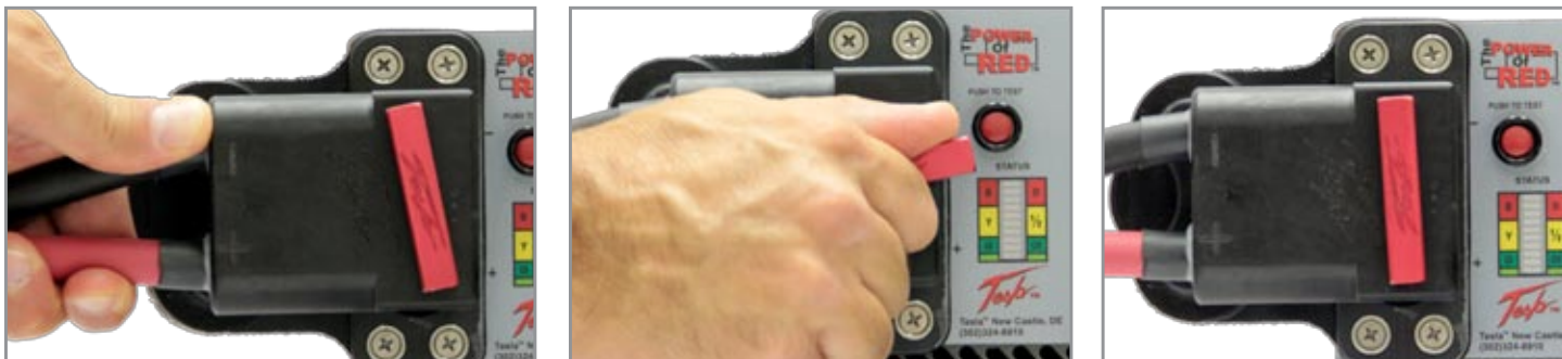
Figure 3.11.1 Attaching DC Power Cable to TI1590 GPU-12
