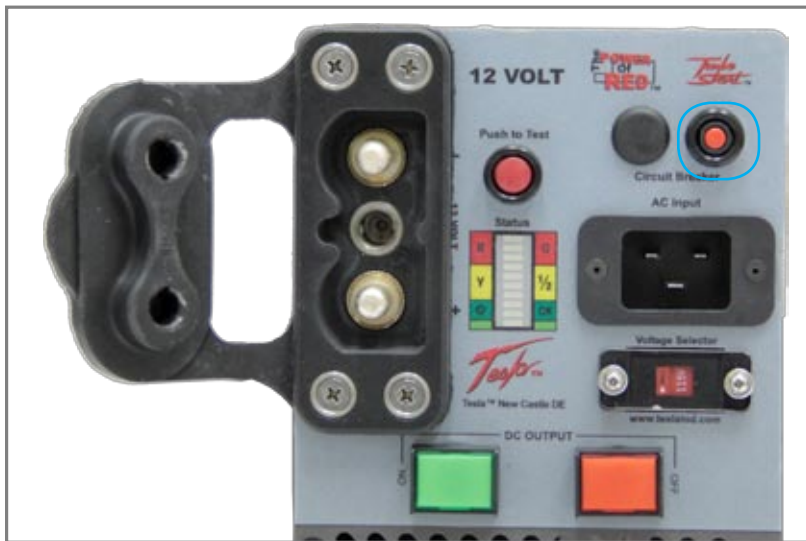
Figure 2.8.1 - AC Input Circuit Breaker (outlined in blue)
